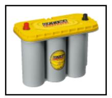
Battery Model: D31A Part Number: 8051-160 Nominal Voltage: 12 volts NSN: 6140 01 502 4973 Description: High power, dual purpose engine start and deep cycle, Pure Lead Absorbed Glass Matt Battery (AGM),
