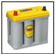
Battery Model: D51 Part Number: 8071-167 Nominal Voltage: 12 volts NSN: 6140 01 523 6288 Description: High power, dual purpose engine start and deep cycle, Pure Lead Absorbed Glass Matt Battery (AGM),
